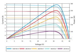
Excellent performance under weak light conditions: at an irradiation intensity of 200 W/m (AM 1.5, 25  $^{\circ}$ C), 95.5% or higher of the STC efficiency (1000 W/m<sup>2</sup>)
